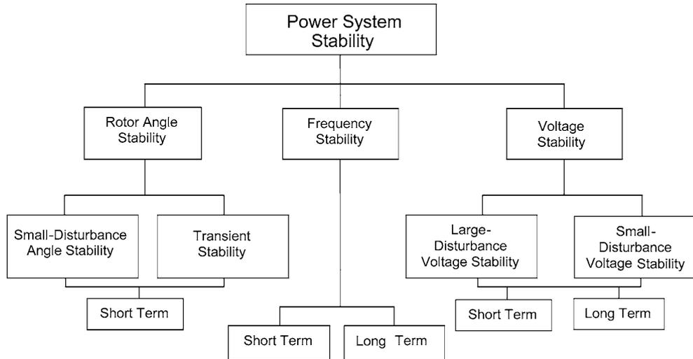
Figure 3-1: Classification of Power System Stability [60]
