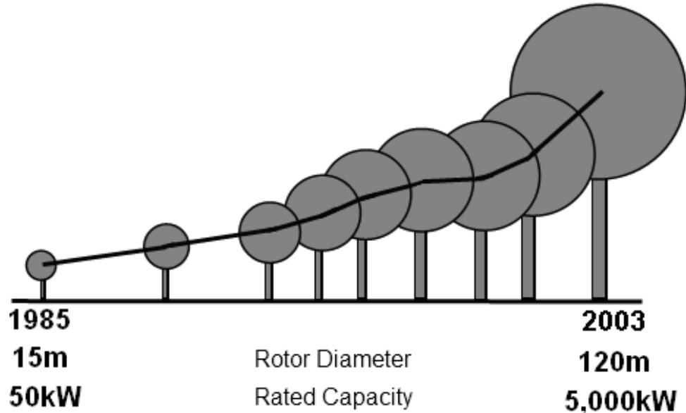
Figure 4-1: Growth in size of wind turbines [28]
