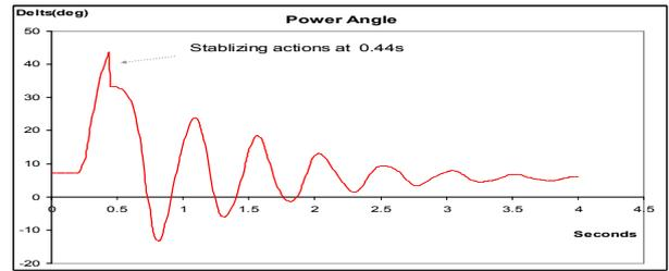
Fig (5) Rotor angle of G1 with control
