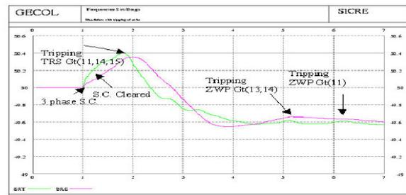
Figure 4 Sequence of events during the first stage
