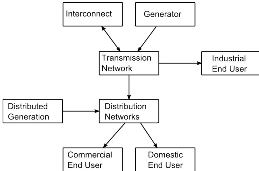
Figure 2-1: Physical Structure of an electric power system
