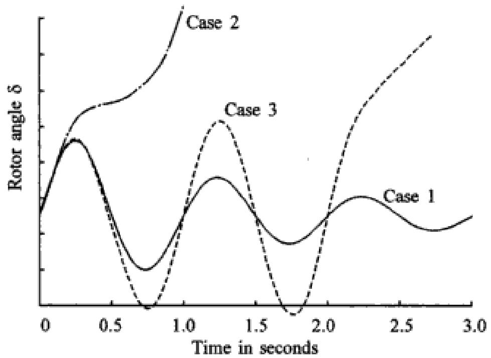
Figure 3-3: Rotor angle response to a transient disturbance [59]
